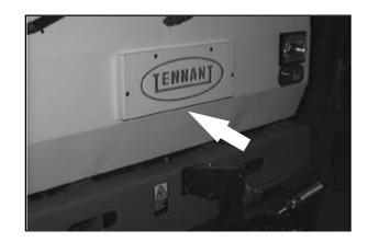
The cab recirculation filter is located on the inside front of the cab in front of the passenger seat. Clean this filter with soap and water.
