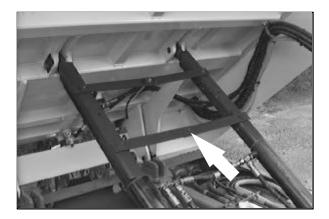
For machine serial number 001710 and above, remove the hopper support pin from the storage location on the right rear fender and place it into the hole of the hopper support cylinder.
