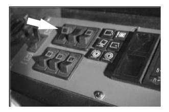
Adjust the amount of water spray to each of the side brushes, with the water valve knobs. Turn the water valve knob clockwise until it comes to a complete stop to close the water supply. If this is NOT done when the machine is shut off, water will continue to flow.
