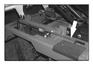
3. Close the vacuum door with the vacuum wand door tool. Place the tool back in its storage location under the hopper.
