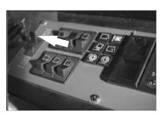
7. Push and hold the hopper lever in the position until the hopper has completely lowered and moved backed into the sweeping position. The hopper tilt light will go off.
