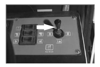
2. Adjust the front angle of the brush, for less angle, and for more angle, with the auxiliary side brush front angle switch.
