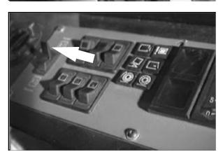
4. Turn the key counter-clockwise. The glow plugs light will come on. When the glow plug light goes out, usually for 5 to 30 seconds depending on the weather conditions, the engine is ready to start.
